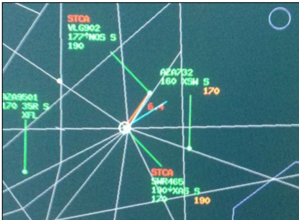
Figure 37 STCA alarm: corrupted SFL
