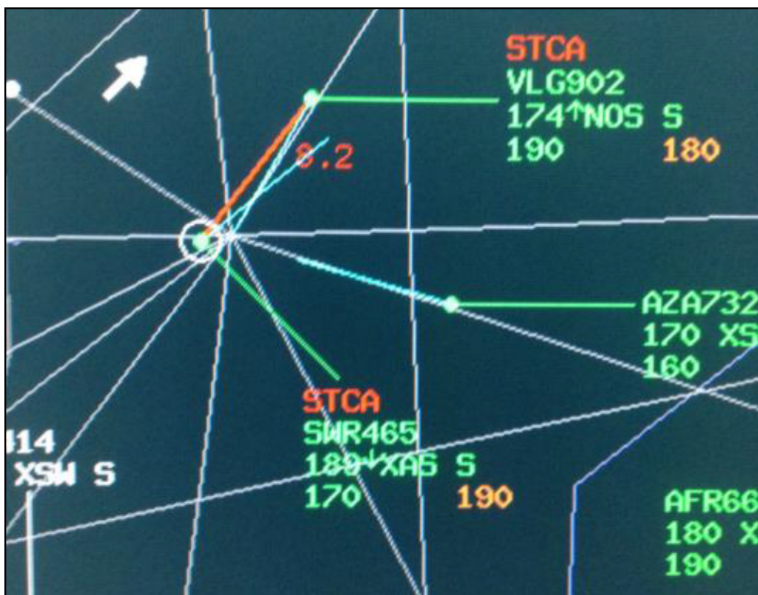
Figure 36 STCA alarm: incorrect MCP/FCU Selected Altitude
